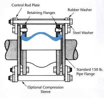
Typical example of a tie rod arrangement. Depending upon size/pressure, two or more rods will be required.
