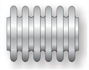
Flexibility of the bellows is achieved through bending of the convolution sidewalls, as well as flexing within their crest and root radii. In most cases, multiple convolutions are required to provide sufficient flexibility to accommodate the expected expansion and contraction of the piping system.
