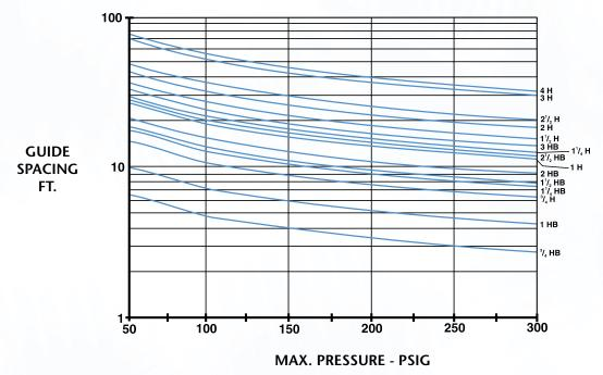
Chart is based upon sch. 40 pipe and type K copper tubing.
