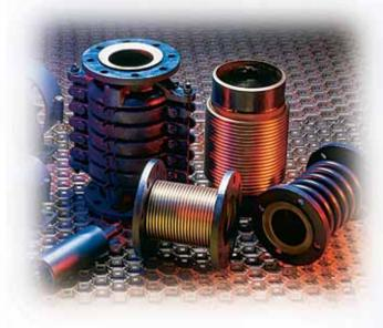
**Exhaust Flexible** Connectors (shown on page 27) are designed for low pressure applications such as stationary and marine gas turbine, diesel engine exhaust, and low pressure ducting. Large motion capability, low spring forces and reduced weight make this product ideally suited for thin-wall duct systems.
