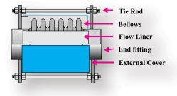
Expansion joints that are installed within ten pipe diameters downstream of elbows, tees, valves or cyclonic devices should be considered to be subject to flow turbulence. The actual flow velocity should be multiplied by 4 to determine if a liner is required per the above guidelines. Actual or factored flow velocities should always be included with design data, particularly flow that exceeds 100 ft./sec. which require heavy gauge liners.
