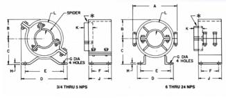
\* For maximum movement, install spider with half its length extended.
